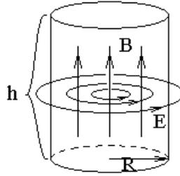
$$\operatorname{rot}(\vec{E}) = -\frac{\partial \vec{B}}{\partial t} \quad \Leftrightarrow \quad \oint_l E_t dl = -\frac{\partial \Phi_B}{\partial t} \quad \Rightarrow$$
